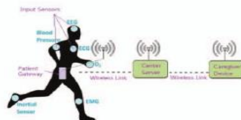
Fig. 1.2 Data monitoring system
