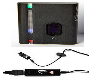
Fig: An emWave2 photoplethysmograph for monitoring heart rate variability, Stone, computer-based photoplethysmograph with ear sensor
