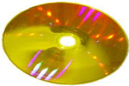
Figure 3: Holographic versatile disc.
