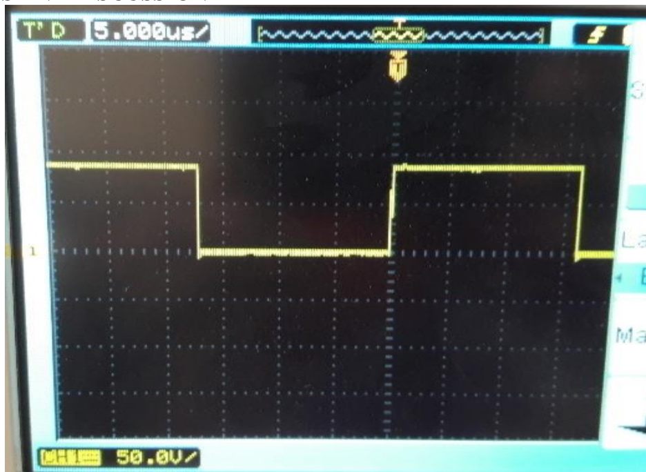
Figure 9: Pulse to drive power MOSFET
