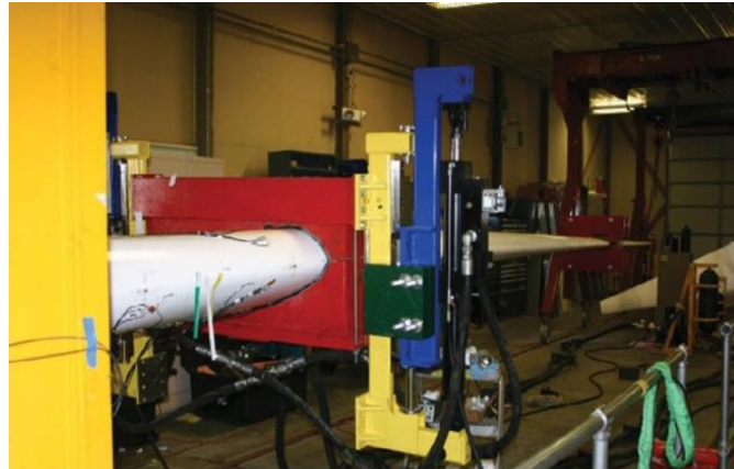
Figure 7: Wind turbine blade experiment under continuous fatigue loading [11]
