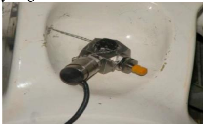
Figure 1: Sensor assembly installation on landing gear [2]
