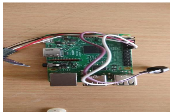
Figure 2: Raspberry pi Board with Buzzer and Zigbee.
