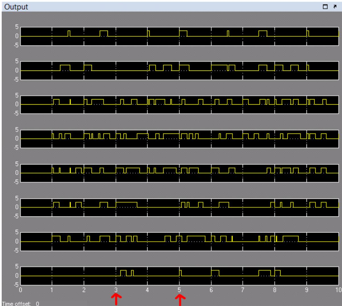
**Fig. 13:** With Time the 8 bit Product  $p_7, p_6, p_5, p_4, p_3, p_2, p_1$  and  $p_0$  Output are Shown from Bottom to Top.
