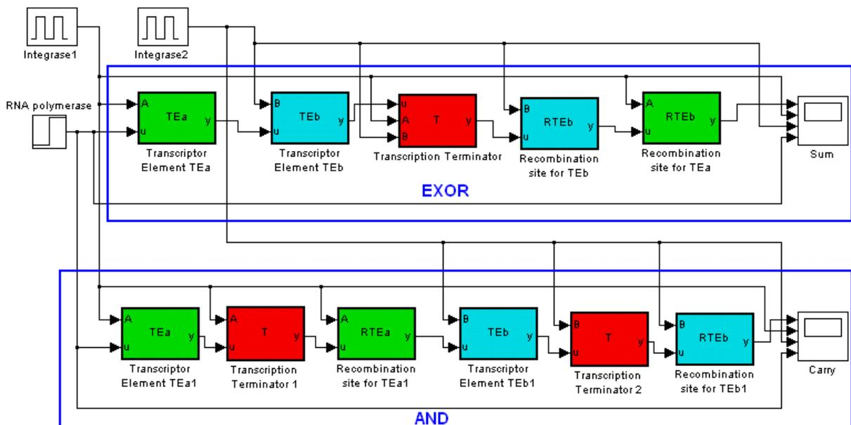
Fig. 9: Simulink Gate Level Design Of Half Adder; TT: Red Color Block, TEs: Green and Blue Pairs.
