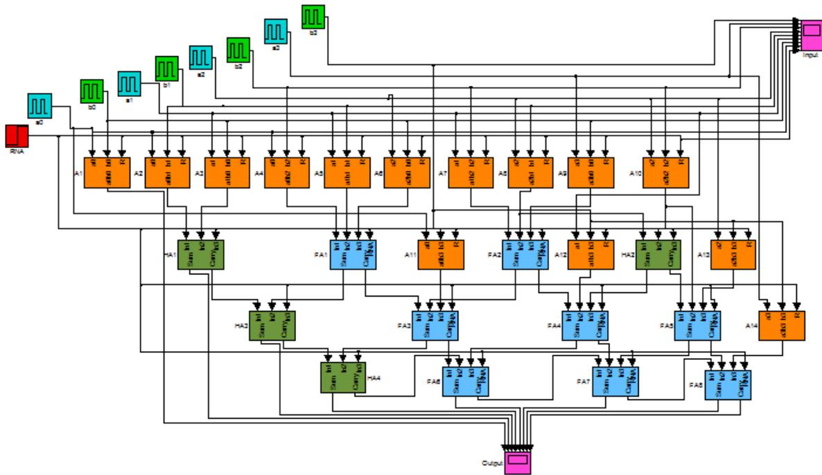
*Fig. 11: Simulink Block Diagram of Wallace Tree Multiplier with 14 and Gates, 4 Half Adders and 8 Full Adders.*
