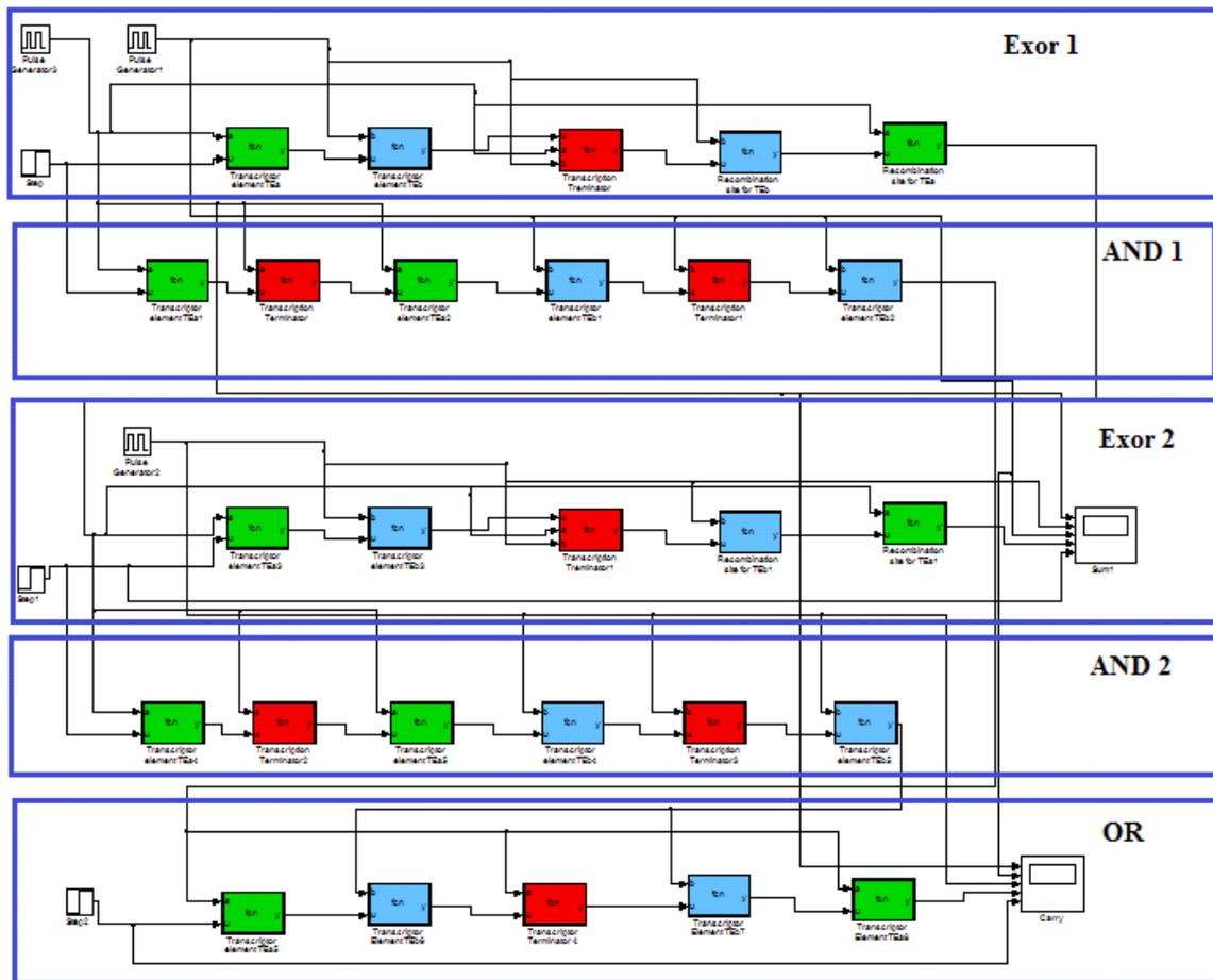
*Fig. 10: Simulink Gate Level Design of Full Adder.*
