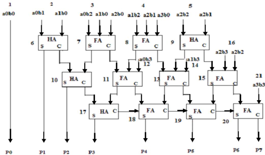
Fig. 3: Schematic for Wallace Tree Multiplier.
