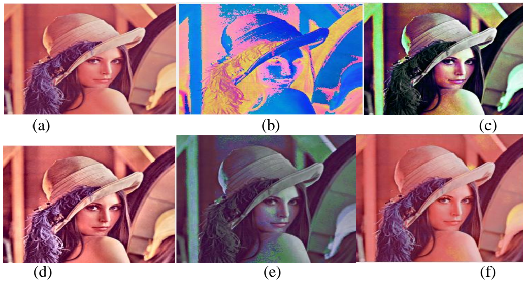
Figure 3: (a) Input image, (b) RGB to HSV, (c) Histogram equalization, (d) Adaptive histogram, (e) Histogram matching, (f) Unsharp masking.
