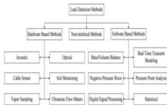
Fig. 2: Classification of Gas Leak Detection Techniques based on their Technical Nature [2].
