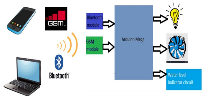
Fig: 1 Basic block diagram of home automation system
