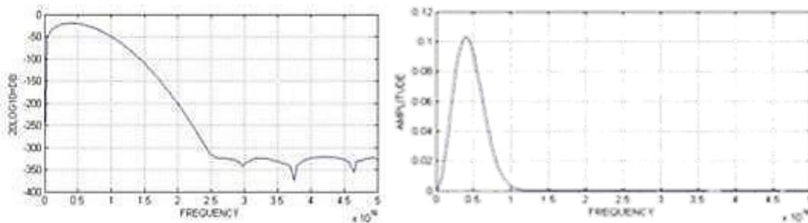
(a) Gaussian Doublet in Frequency Domain (b) Magnitude Spectrum of Gaussian Doublet
