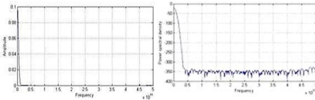
(a) Gaussian Pulse in Frequency Domain (b) Magnitude Spectrum of Gaussian Pulse
