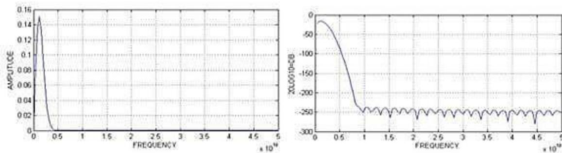
(a) Gaussian Monocycle in Frequency Domain (b) Magnitude Spectrum of Gaussian Monocycle
