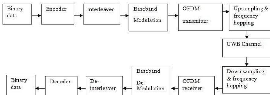
*Fig 8. Block diagram of UWB OFDM system [15]*
