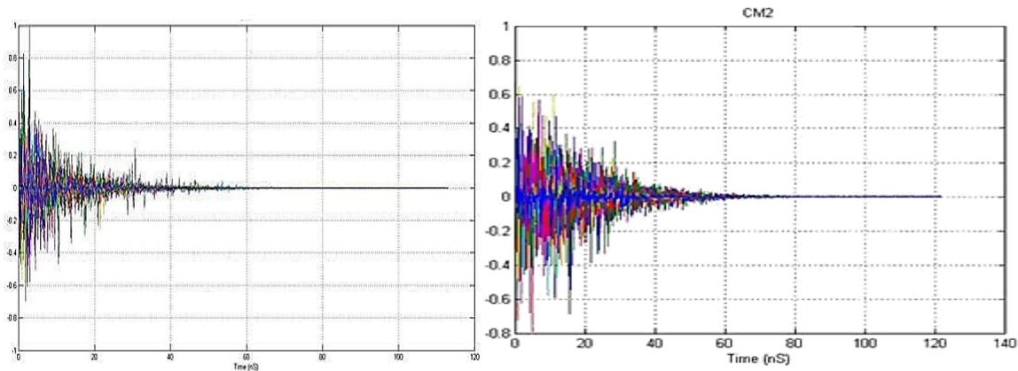
(a) Impulse response realization of CM1 (b) Impulse response realization of CM2
