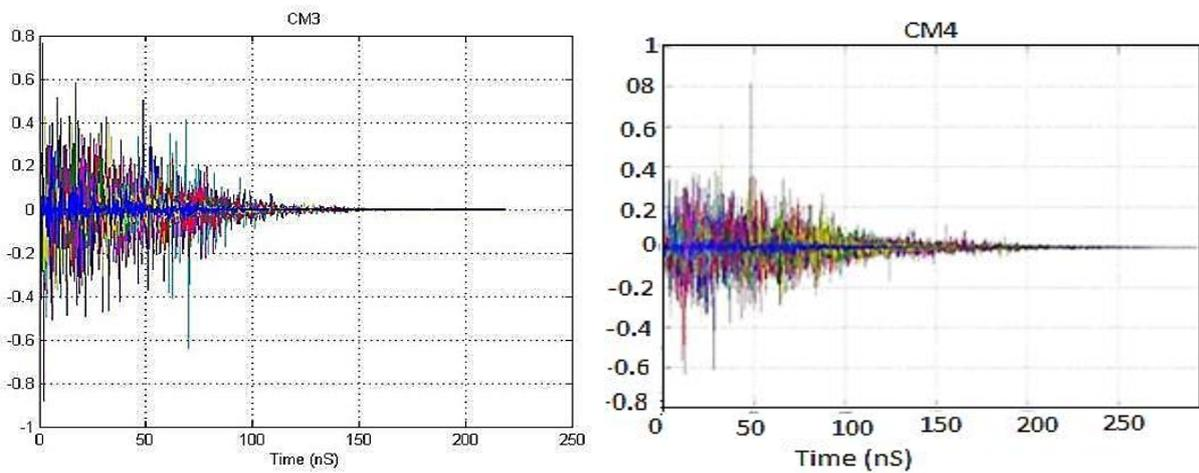
(c) Impulse response realization of CM3 (d) Impulse response realization of CM4
