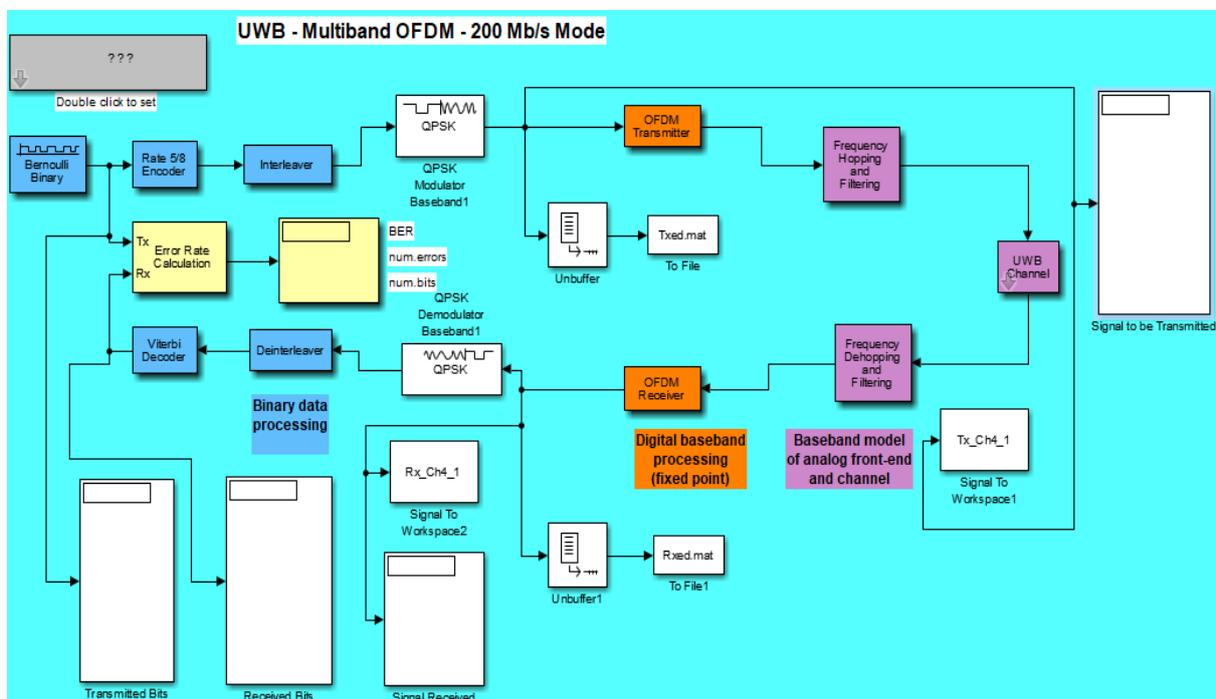
*Fig 9. UWB OFDM simulink model implemented in MATLAB*
