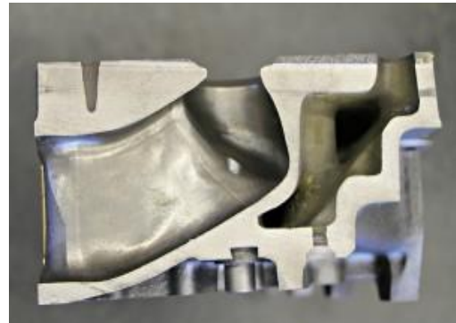
Fig. 1 Cylinder head Air passage and Coolant passage
