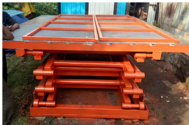
Fig. 4 Actual Photo, Scissor type car lifter
