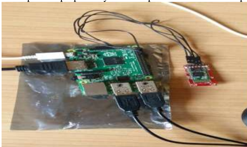
Fig.2 Bluetooth module acting as interface between Raspberry Pi & mobile
