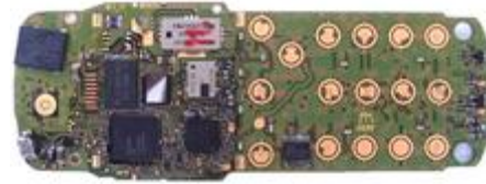
Fig 1.2: A printed circuit board inside a Nokia 3210
