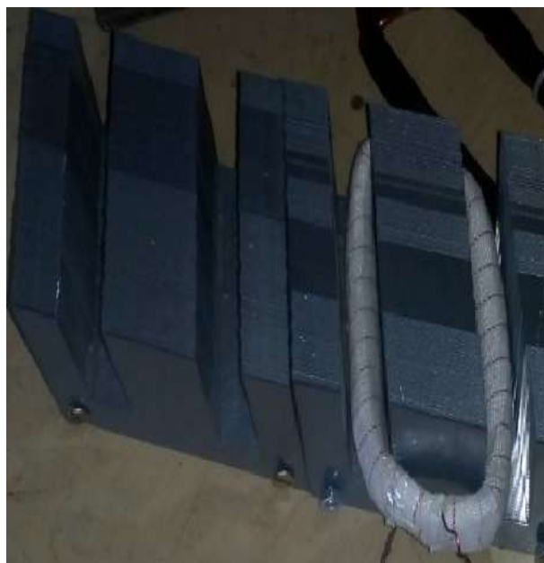
Fig. 6: Assembly of Stamping with Coil.
