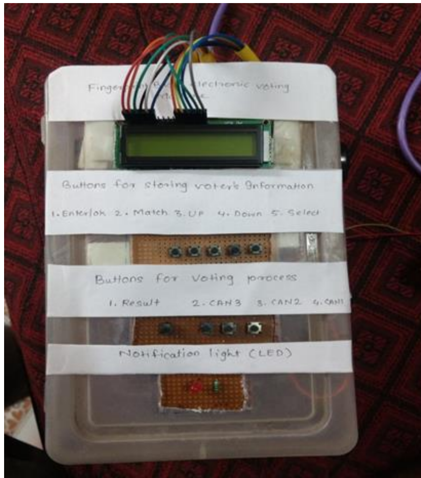
Figure 3: Electronic voting machine using fingerprint
