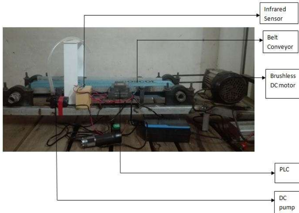
Figure 6: Final Construction of an automatic bottle filling machine
