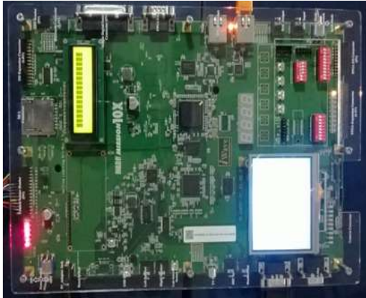
Fig. 2: Spartan 6 FPGA with OMAP.
