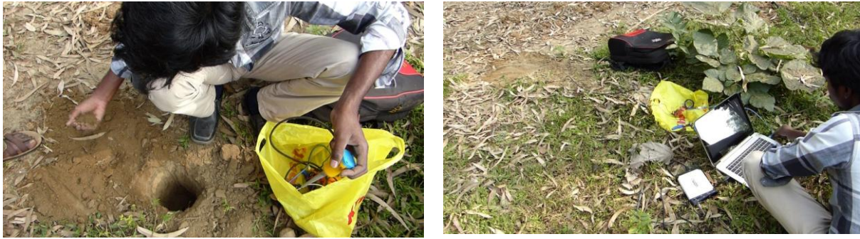
Fig. 4: Outdoor Field Testing of GVSSID System; Sensor Placed 30 cm Underground (Left) and System Under Operation (Right).
