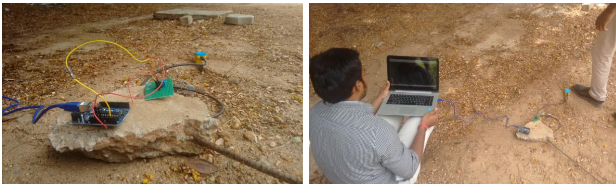
Fig. 5: Field Testing of Horizontal Geophone based GVSSID with Human Footsteps: System on Operation (Left) Footstep Input (Right).
