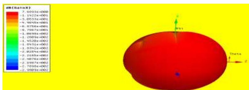
Fig. 2: Polar Plot (Gain) of Conventional Patch Antenna.
