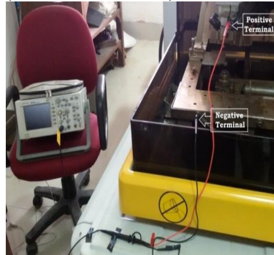
Fig 3: oscilloscope connection by passive probe to the two (positive/negative) terminals
