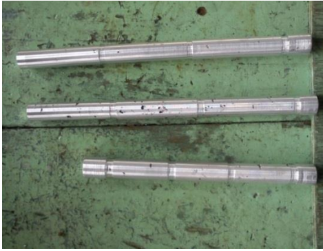
Fig 1 Sample for surface roughness test
