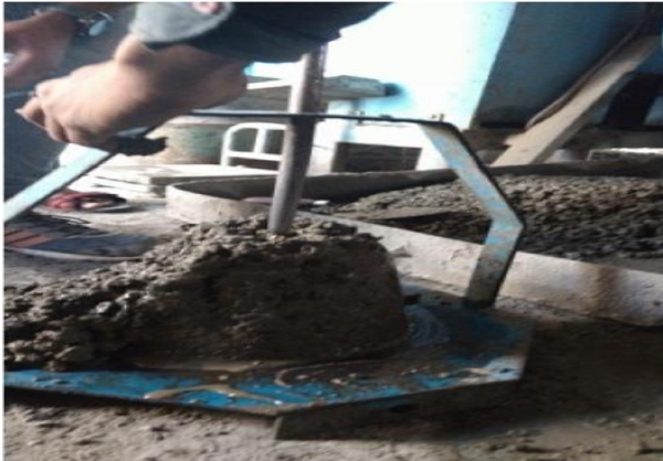
Fig. 2 Slump Showing the workability of Concrete
