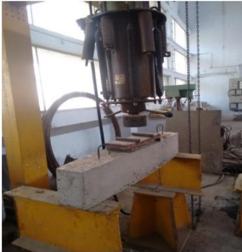
Fig. 5. Loading arrangement of beam
