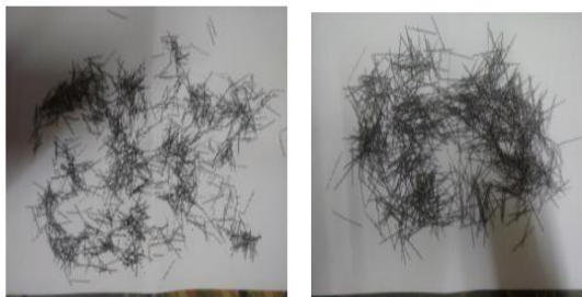
Fig. 3. Steel fibers of aspect ratio 30 and 60
