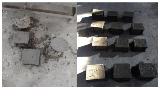
Fig. 2. Casting of specimens
