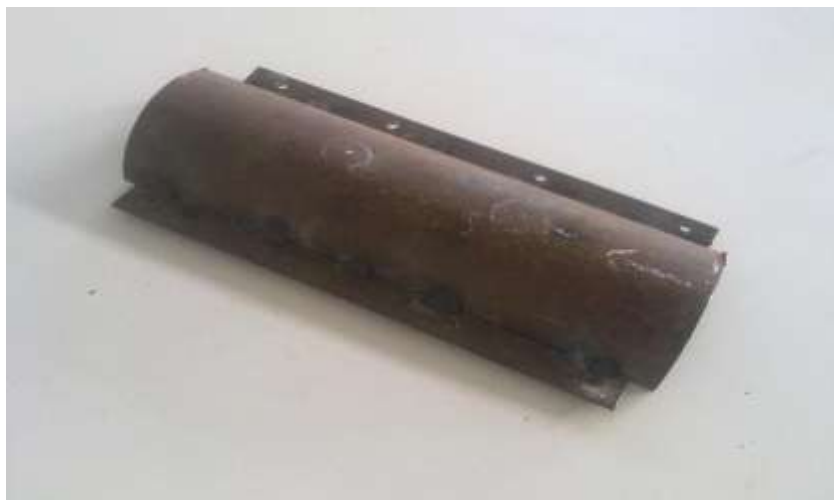
Fig. 3: Drilling of collars for making holes of nut & bolts.
