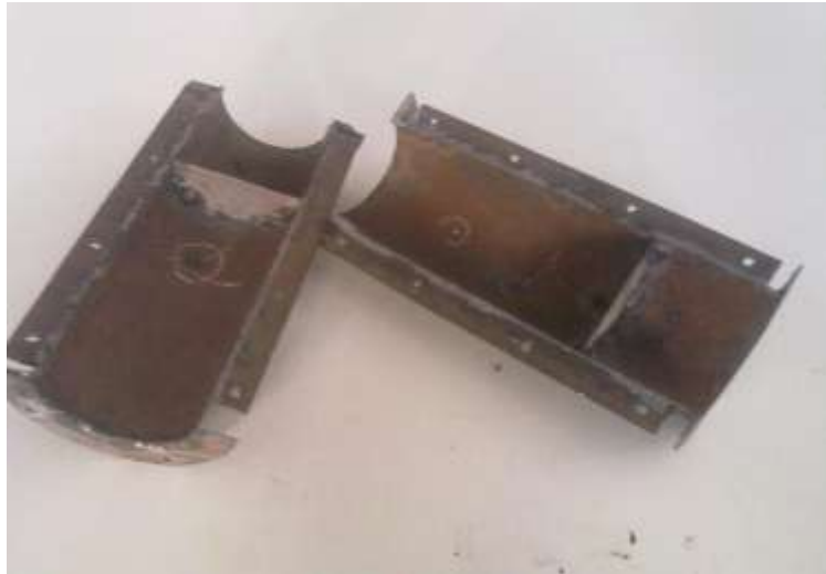
Fig. 5: Welding of semi - circular plates.
