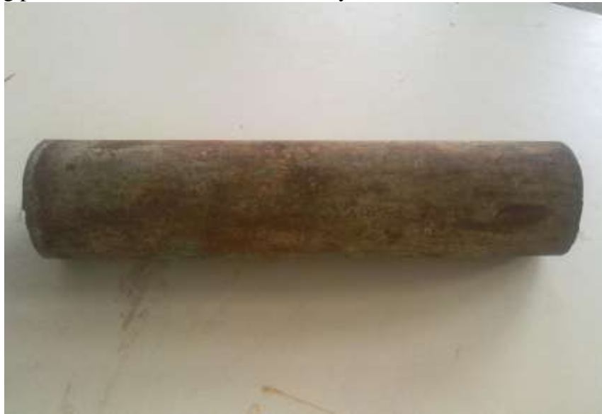
Fig. 2: Cutting of 4-inch diameter M.S. Pipe in lateral direction.
