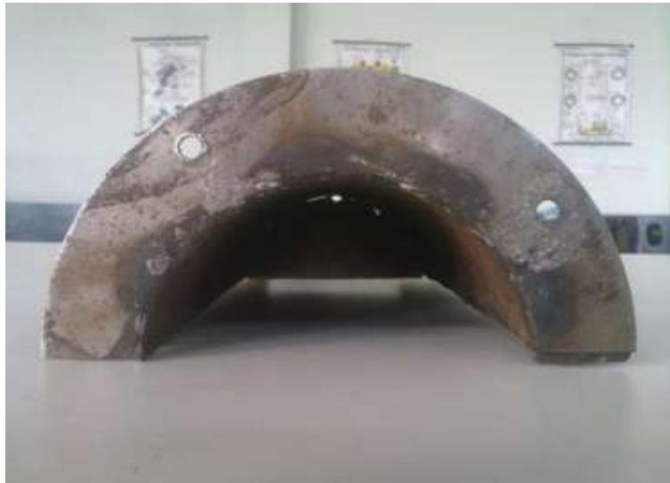
Fig. 4: Welding of collars on the semi - circular pipes.
